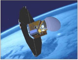
at 280-800nm and an IR channel at 1.27 microns. In astronomy mode it uses a radiometer working at 486-580 Ghz and 119 Ghz. Both modes use the satellites 1.1m telescope in a 3-axis stabilized mode. The satellite can switch back and forth between modes on the fly.
