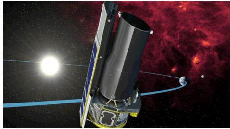
Like the Gaia spacecraft, the Spitzer telescope is not in earth orbit. It is in an earthtrailing orbit around the sun with an eccentricity of .011, a perihelion of 1.003AU and an aphelion of 1.026AU. It is inclined to the ecliptic by 1.13 degrees and has a period of 373.2 days.
