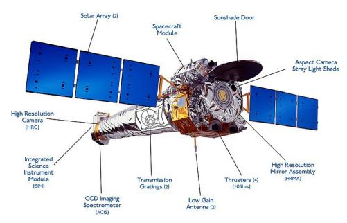
As X-rays can't be focused by a normal mirror, the Chandra satellite uses a series of 'grazing incidence reflectors' which look like slightly curved cylinders. The X-rays hit these at a slight angle and are reflected into the next, and the next etc. Until they come to focus at the sensor
