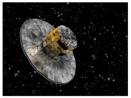
The spacecraft has a mass of just over 2t and its dimensions are 4.6m x 2.3m. It is solar powered with a circular array that generates over 1.9kW. It was boosted by a Soyuz ST-B/Fregat-MT rocket from Arianespace's facility at Kourou.
