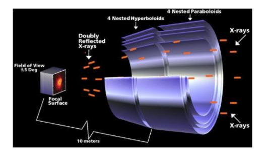
The spacecraft isquite as the focal length of the reflectors is 10m and its mass is 5.9t. The telescope has a collecting area of .04 square meters and operates from .1 to 10keV and has a resolution of .5 arcsec. Its planned 5 year mission has been extended and it is currently approaching 20 years in operation.
