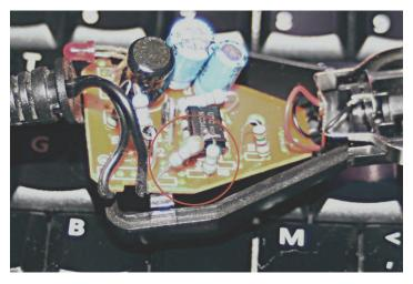
In the image to the left you can see the two 3.9K resistors standing up and soldered together. The original 1.5K resistor is just to their right.
