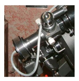
The ST-4 was available with a dedicated flip-mirror and reticule eyepiece that was very nice. The reticule showed a rectangle that equated to the field of view of the sensor which made things very simple.
