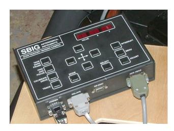
especially when it's hot outside. The unit allows the taking of a dark-frame which will keep hot-pixels and other thermal noise to a minimum. When used correctly the ST-4 can guide to within 1/5 of a pixel which is very accurate.
