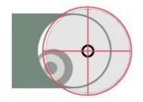
Now place your Cheshire sight tube in the focuser (red). If you are using a 2" to 1.25" adaptor then orient the adaptor so that its tensioning thumbscrew is opposite the one that is holding it in the focuser. Look into the tube and adjust the three (or four) collimating screws on the secondary so as to put the cross-hairs on the primary mirror's centre spot. The grey circle is the shadow of the secondary and Chesire.
