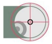
The next step is to put your sight tube back in the focuser and readjust the secondary to put the cross-hairs back on the centre spot (things may have shifted when you centred the secondary). Illustration 4. With the Cheshire in place adjust the primary mirror's adjustment screws or knobs until the shadow of the secondary and Cheshire are under the cross-hair. Don't worry if the shadow of the secondary is off centre. It is supposed to be.
