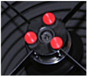
the dark, in the field, is a recipe for catastrophe. On receiving the telescope I replaced the screws with M4 screws with press-on knobs from the local fastener store. These work perfectly and I'm not tempting fate when setting collimation.
